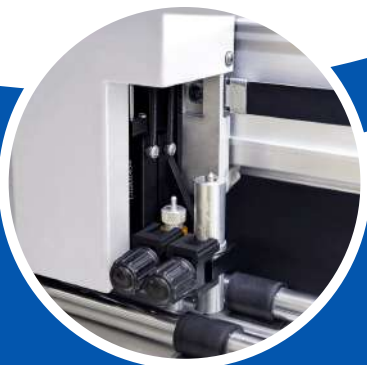
Double Knife Head Design Die-cutting + Indentation
